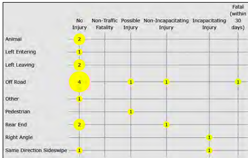
Figure 10. Crash type vs. severity on CR-280 from SR-73 to SR-71
